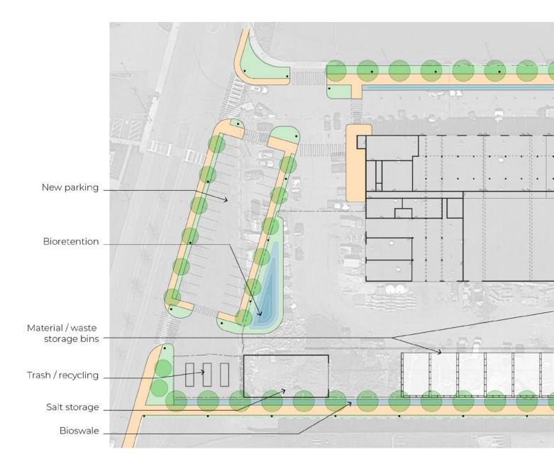
This detailed site plan shows the new parking configuration at the Commercial Street entrance with an adjacent bioretention basin to capture runoff from the western areas of the site. Two bioswales on the north and south carry stormwater runoff to bioretention areas closer to the river. Within the DPW yard, new precast concrete block storage bins organize
