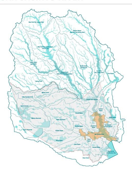
The designated San Jacinto River watershed includes the San Jacinto River downstream of Lake Houston as far as the Baytown bridge, where it flows into Galveston Bay, as well as the Houston Ship Channel. HCFCD has built detention on side channels of the Ship Channel. The river itself, though, is managed by the San Jacinto River Authority, which operates the dam on Lake Houston. The river's floodplain south of the dam includes residential areas which have flooded repeatedly.
